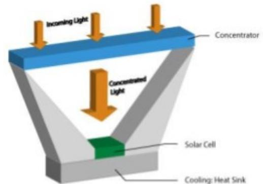
CPV involves concentrating a large area of sunlight into a small solar cell, thereby increasing panel efficiency in given surface area.
