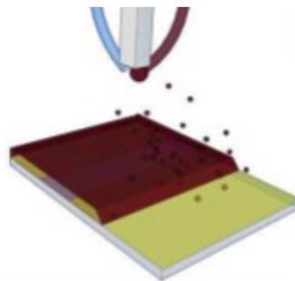
Spray-coating methods, coupled with perovskite film cells, can be used to produce cheap solar panels.
