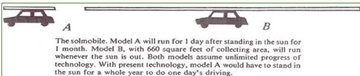
The above diagram, produced 30 years ago by Petr Beckmann, professor of electrical engineering, clearly demonstrates the inefficiency of traditional silicon-panelled solar power. The time that has passed since the creation of this diagram has not changed the situation – it is
