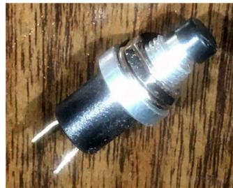
The switch is a center off type switch. This is also referred to as On - Off - On. The center off switch allows both the solar panel and the batteries to be disconnected. This is useful when there is intermittent or weak sunlight. The solar panels can be disconnected and they don't have to be covered and the batteries won't be drained unnecessarily.
