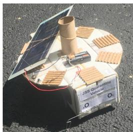
This photo is the JSS Quarantine Vehicle. Its chassis was fabricated primarily from the solar panel shipping box. Following this are close up shots of the battery system controls. These are shown alongside the schematic diagram of the battery circuit. The intent is to facilitate the student's fabrication of the battery circuit.
