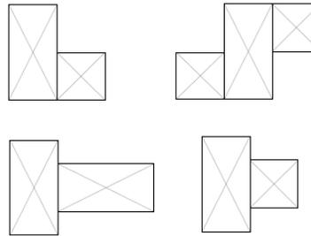
3. Lap joints are allowed and involve gluing two pieces of basswood material with the grain pattern normally at right angles; however, any lap joint less than  $10^\circ$  or greater than  $170^\circ$  would circumvent the lamination guidelines and will be ruled unacceptable.
